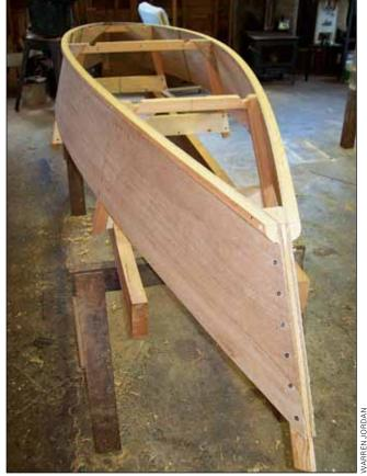
Marine plywood panels (¼" or 6mm thick) make up the sides, and then chine logs (long strips along the boat's bottom) are attached to the outside of the hull. A plywood bottom will cap the assembly.
